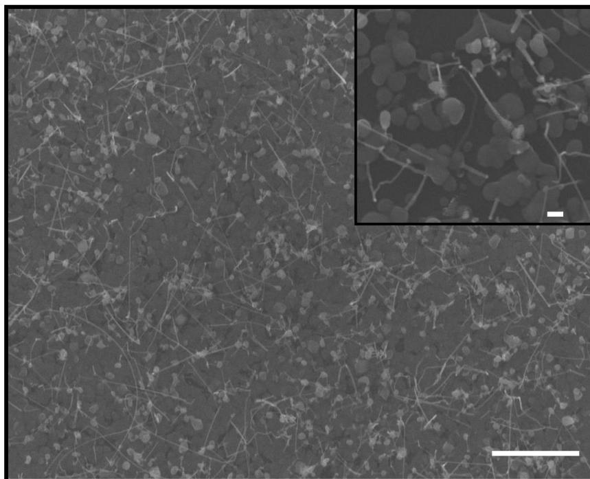
**Figure 1:** FESEM image of Ge nanowires and inset is corresponding magnified image. The scale bars of low and high magnified images are 1 μm and 100 nm, respectively.
