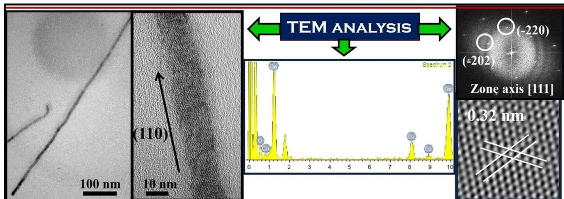
**Figure 2:** (a) TEM image of the germanium nanowire and corresponding, (b) EDS spectrum (c) SAED pattern and (d) HR image. The scale bars for (a) and (b) are 100 nm and 10 nm, respectively.
